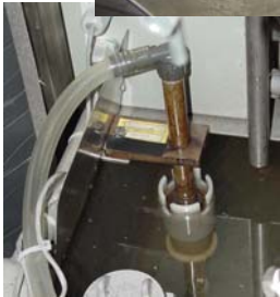
Mini Coalescor installed on a JENFAB LeanClean 360 Rotating Basket Cell Washer
