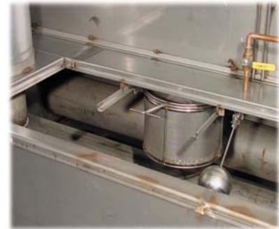
View of exposed drum. Top of drum enclosure and drum are easily removed
