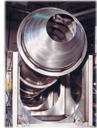
View of exposed drum. Top of drum enclosure and drum are easily removed
